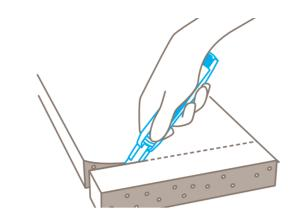
**Depending on your cutting job** leave your thumb at first on the slider to fix the blade.
