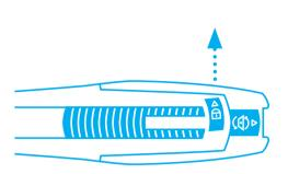
To lock the slider shut, **push the safety device** upwards as marked by the arrow.
