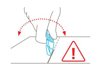
If the blade head gets stuck, **don't forcefully lever** the knife!
